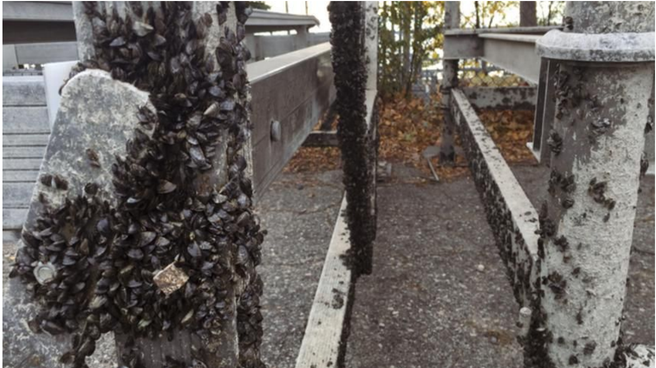
(Boat lifts removed from Green Lake, 2015, second year of zebra mussel infestation - West Central Tribune.)
